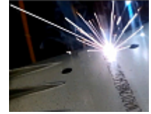
Automotive VIN Marking
